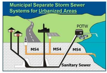
Figure 9: A diagram of an MS4 system.
